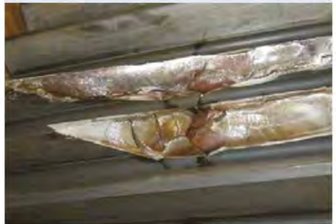
Figure 2 Overload breakage on a tooth flank
