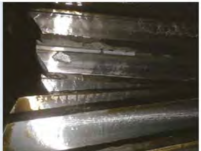
Figure 8 Visible corrosion at the tooth flank
