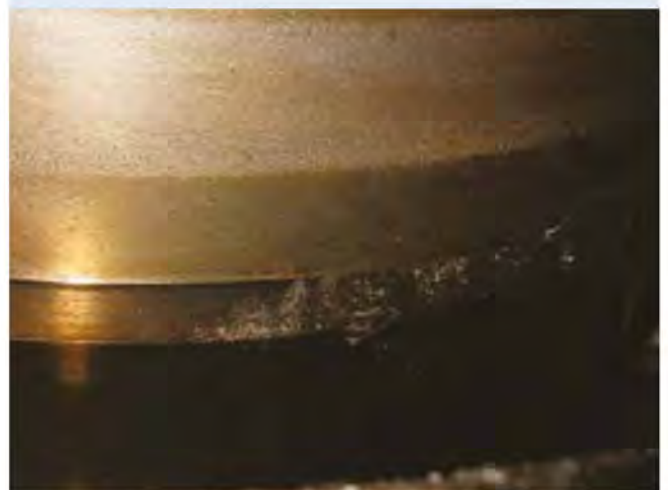
Figure 9 Surface fatigue phenomena on a bearing ring
