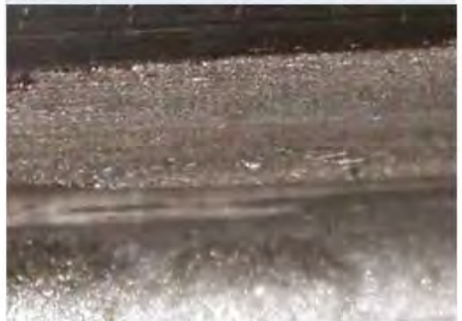
Figure 7 Tooth flank with micropitting and corrosion
