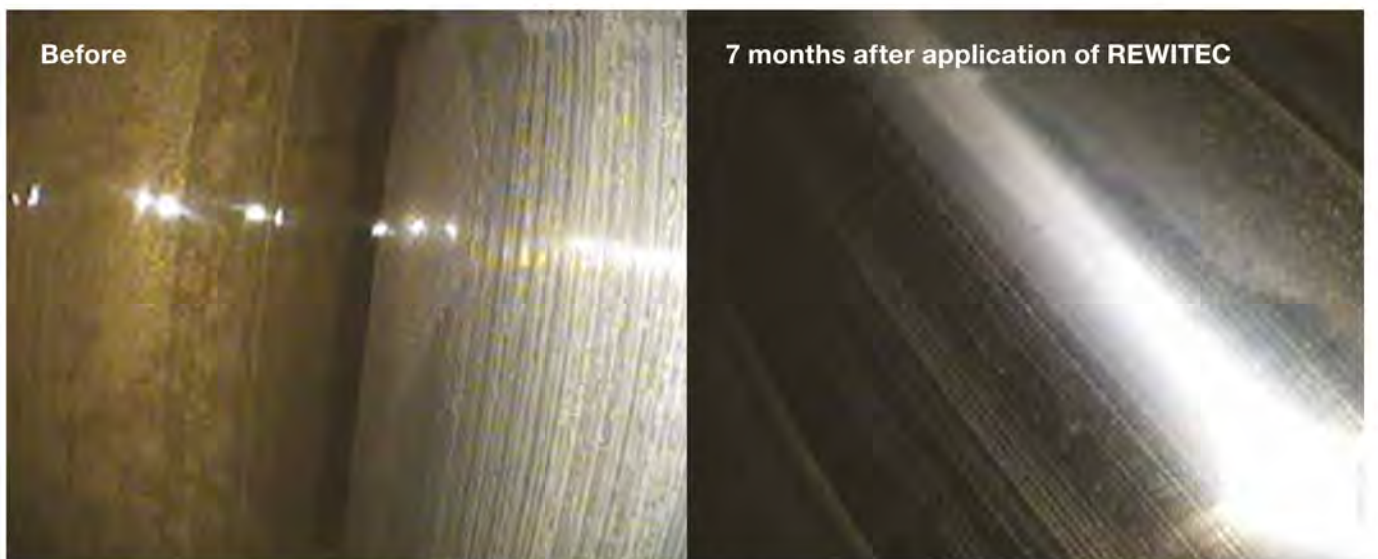
Figure 16 Surface grooves at planetary bearing before and after the application of REWITEC
