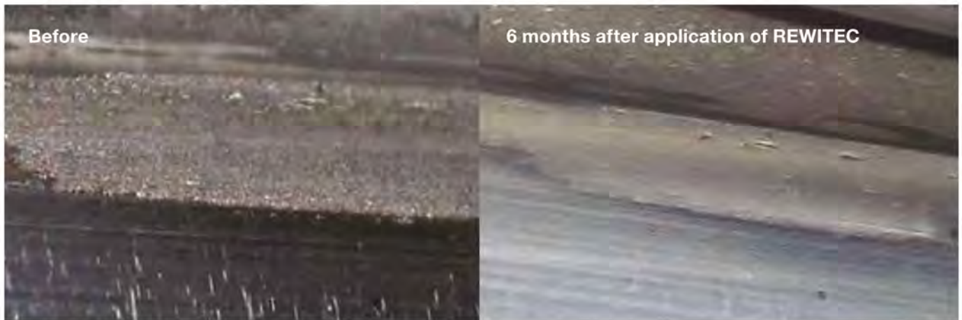
Figure 14 Micropitting and corrosion before the REWITEC application
