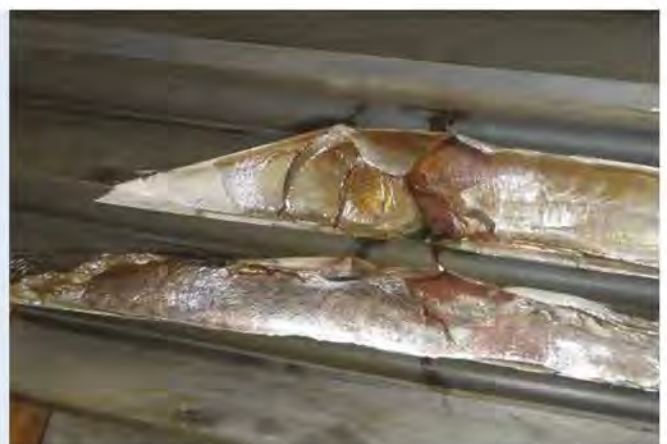
Figure 3 Overload breakage on a tooth flank
