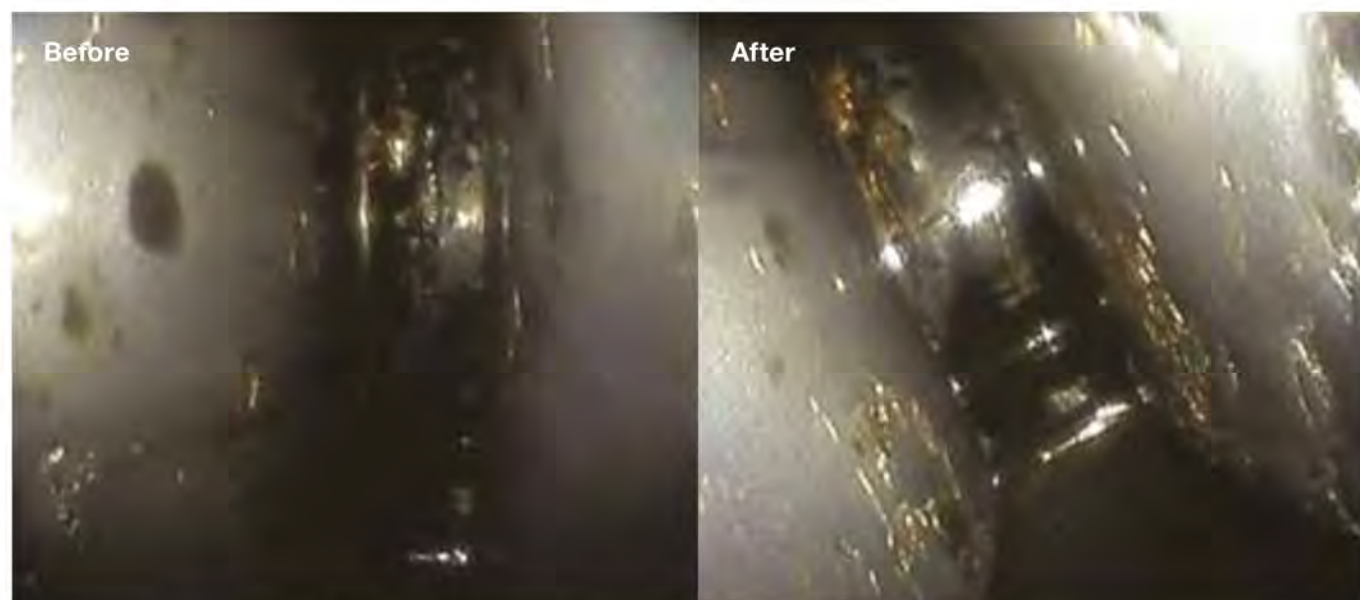
Figure 18 Rolling element in a planetary bearing, before and after the application of REWITEC
