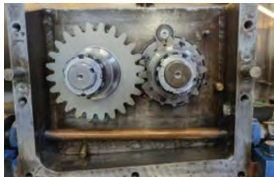
The FZG test was used to assess the operating temperature over the different load stages.
